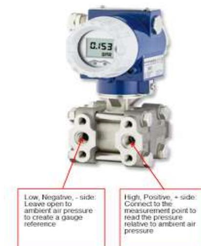
through the signal cable or a hole beside the electrical connector. So by leaving the negative side port of the differential pressure sensor vented to atmosphere, you are in effect creating a gauge reference pressure sensor.
